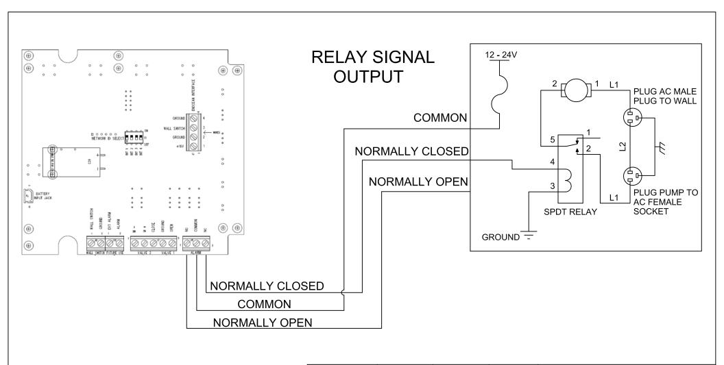
RS-360 Wiring Schematic: Dry Signal Contact Wiring to a Plug-In Relay
