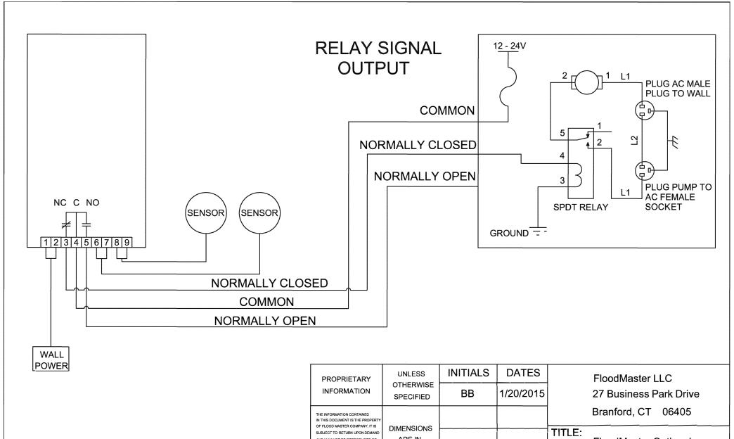
Wiring Schematic for RS-080, RS-092, RS-094, and RS-096 Dry Signal Contact Wiring to a Plug-In Relay
