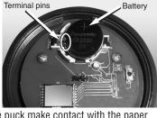
Insert battery UNDER the terminal pins on the left side of battery holder
